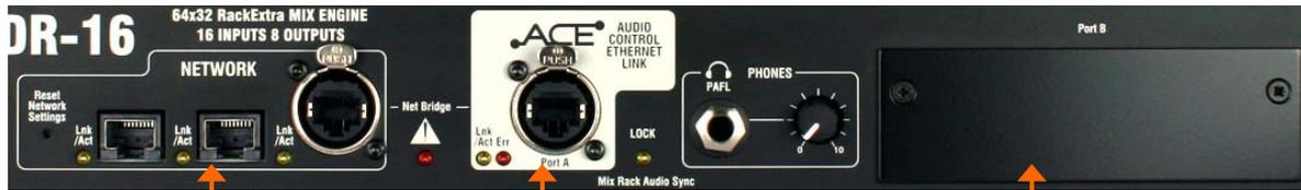
**Control network** 3 port Ethernet switch. Connect laptops, wireless router, link iLive networks, connect external TCP/IP networks, or link to an iLive Surface that does not have an ACE™ port. Control only, no audio.
