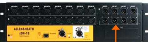
**xDR-16** I/O expander rack adding more input and output sockets plus a Port B card slot. Requires ACE™ fitted to MixRack Port B.
