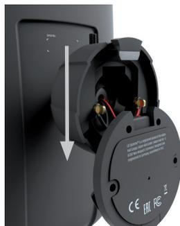
**2** Firmly secure the wall mounting plate with the terminal block at the top using suitable screws on a wall sufficiently capable of supporting the load. For speaker cables laid under plaster, the corresponding cable must be inserted through the central cable bushing prior to securing the wall mounting plate. Now connect the speaker cables to the corresponding contacts of the terminal block.
