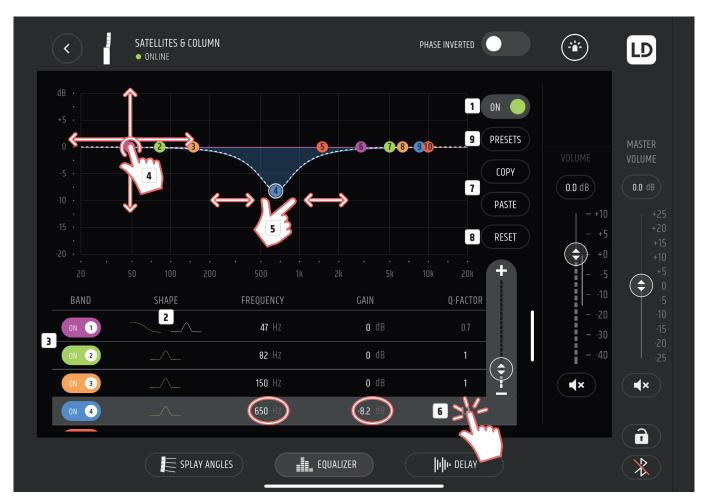
The EQ settings can be stored in seven individual presets and recalled later. Tap PRESETS **9**, then tap the desired empty slot **10**, tap SAVE **11**, enter the desired name for the preset and confirm the entry by tapping Done **12**. To cancel the procedure tap on Cancel.
