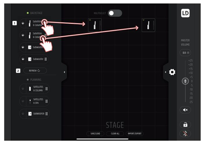
With offline devices, you can plan your stage and save and load it using the SAVE/LOAD button. To link ONLINE devices with your pre-planned STAGE, simply drag and drop the ONLINE devices onto your planned offline devices on stage. To remove devices from the STAGE, you can drag and drop them back into the device list or select them and tap the delete button in the settings column on the right.
