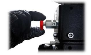
3.- Once the telescopic is fully lowered, turn the safety bolt knob to the position with the arrow pointing to the left:
