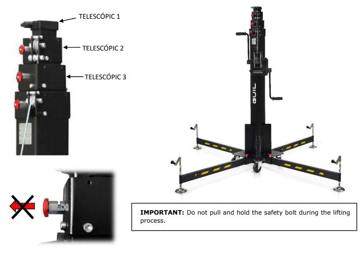
3.- Repeat these steps to raise the remaining telescopic sections (telescopic 2 and then 3) until the tower is at the desired height. You should hear the safety bolt clicking into each safety hole as the telescopic masts are extended.
