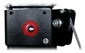
1.- Turn the safety bolt knob blocking the first section (telescopic 1) to the position with the arrow pointing to the right.
