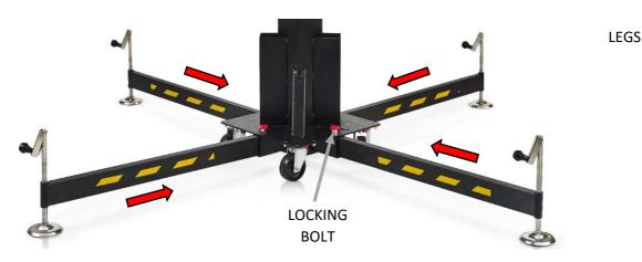
4.- Level the tower by adjusting the levelling jacks of the stabiliser legs and using the spirit level located on the mast as a reference.
