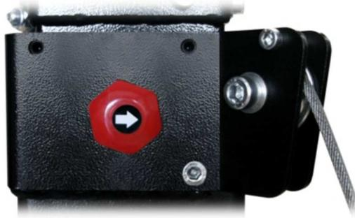
2.- Pull and hold the safety bolt in this position and turn the winch handle lowering the telescopic section.
