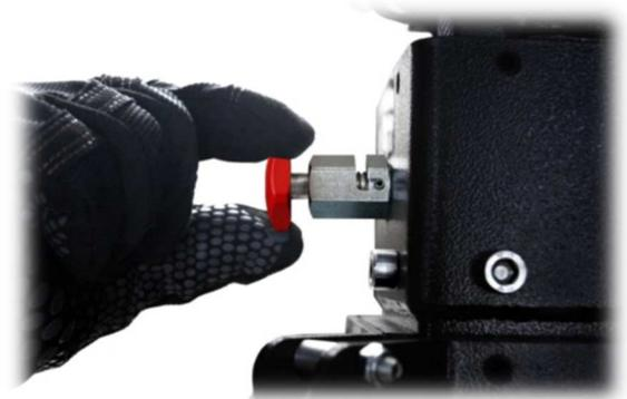
3.- Once the telescopic is fully lowered, turn the safety bolt knob to the position with the arrow pointing to the left:
