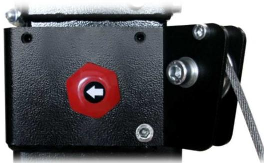
1.- Turn the safety bolt knob blocking the first section (telescopic 1) to the position with the arrow pointing to the right.
