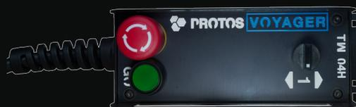
Optionally a remote control is available in either handheld or wall mounted iterations and comes with a standard 20m cable. The variable speed TW is controlled through the PVC-TW01RVS a single channel, 19 inch rack mount which features speed control and an E-switch. It can be programmed with the use of a PC or tablet which can be connected with a TJ 45 LAN or DMX connection to the controller.
