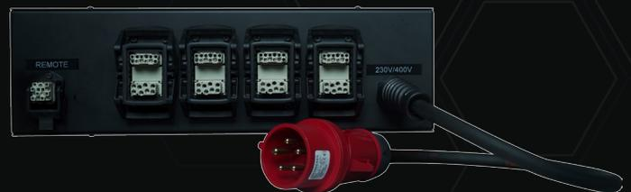
The fixed speed TW model is controlled via the PVC-TW04R 4 channel or the PVC-TW 01R 1 channel controllers. These controller has up/down switches for each channel and an E-stop switch. Controllers can be linked with up to a maximum of 24 units (96 channels) and are equipped with Harting and CEE 16A connectors. They can also be equipped with a DMX 512 show control card.
