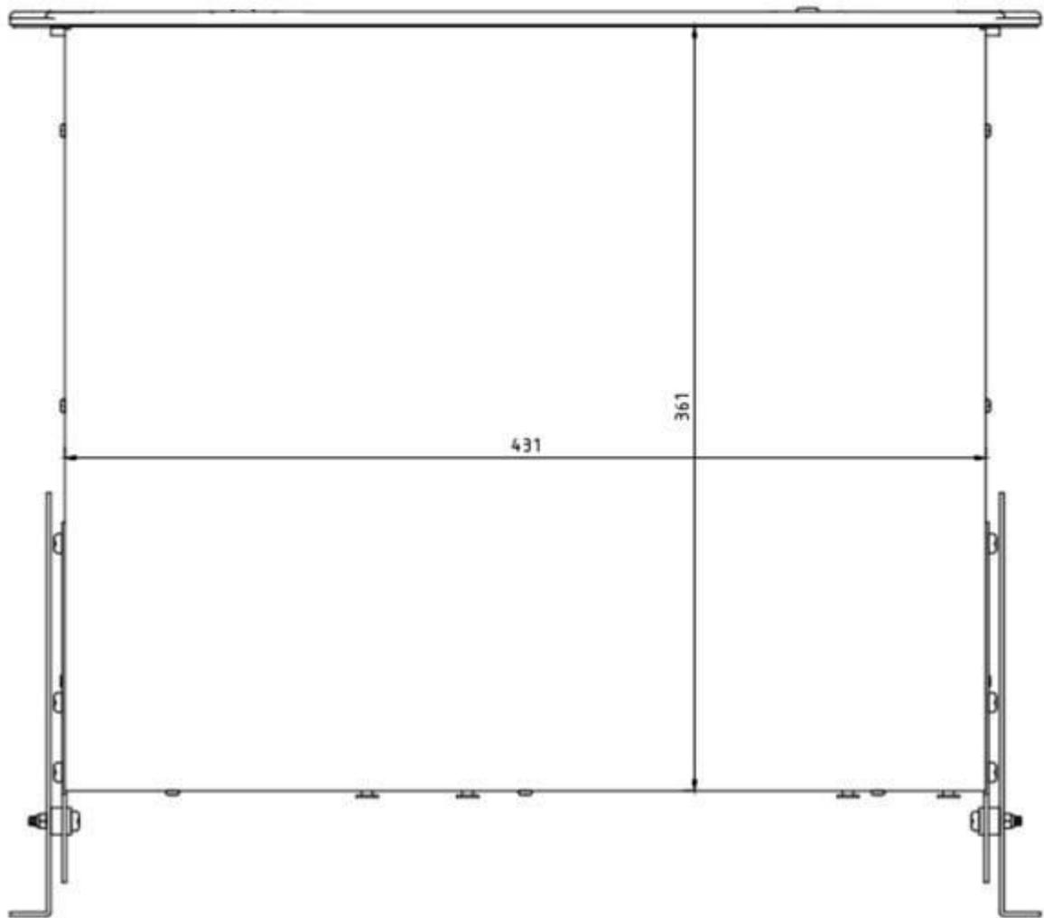
The C3 DSP amplifier system is designed to be mounted in a standard 19" rack enclosure.
