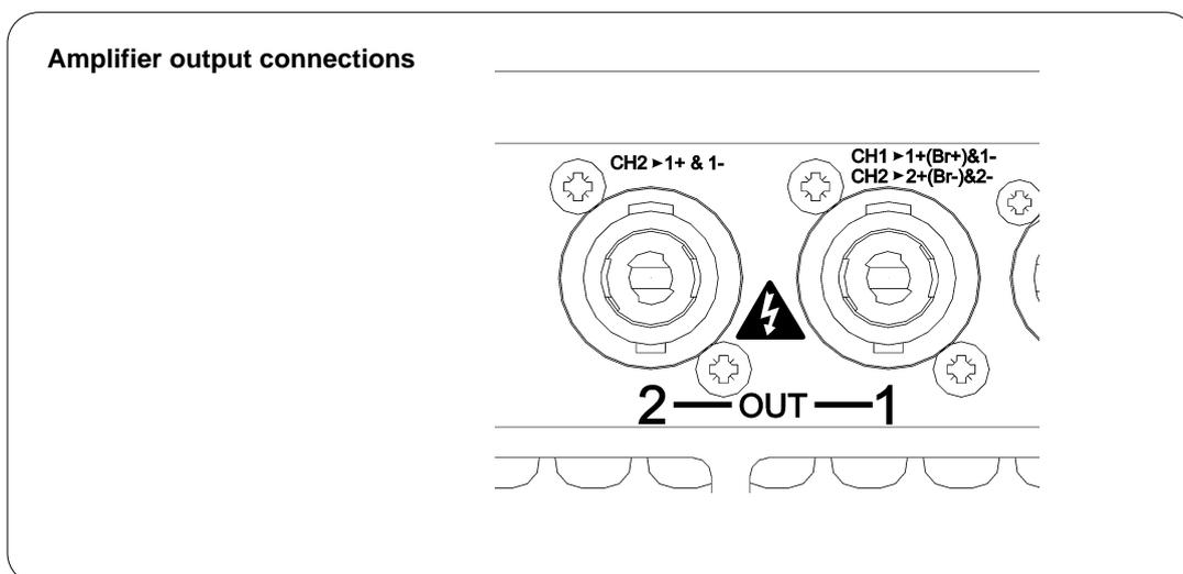
The Speakon™ connector for amplifier channel 1 carries the output for amplifier channels 1 and 2. In addition this connector can also be used if the pair of amplifier channels is being operated in bridged mode.
