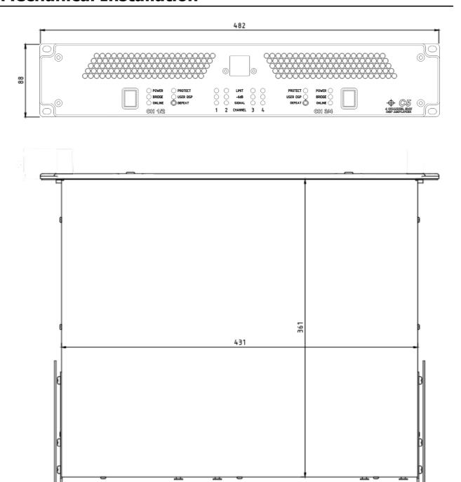
The C5 DSP amplifier system is designed to be mounted in a standard 19" rack enclosure.
